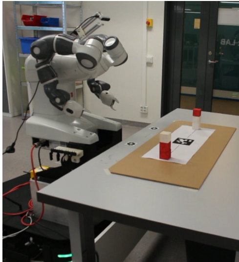
(a) The mobile manipulator at the workcell where it has to build a pyramid with blocks.
