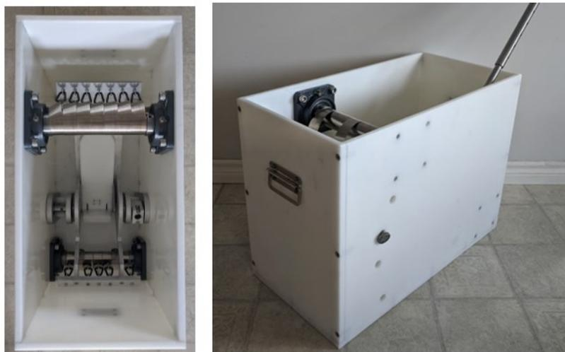
*Figure 3.3 : View of the assembled device. A) Inside and B) and outside.*
