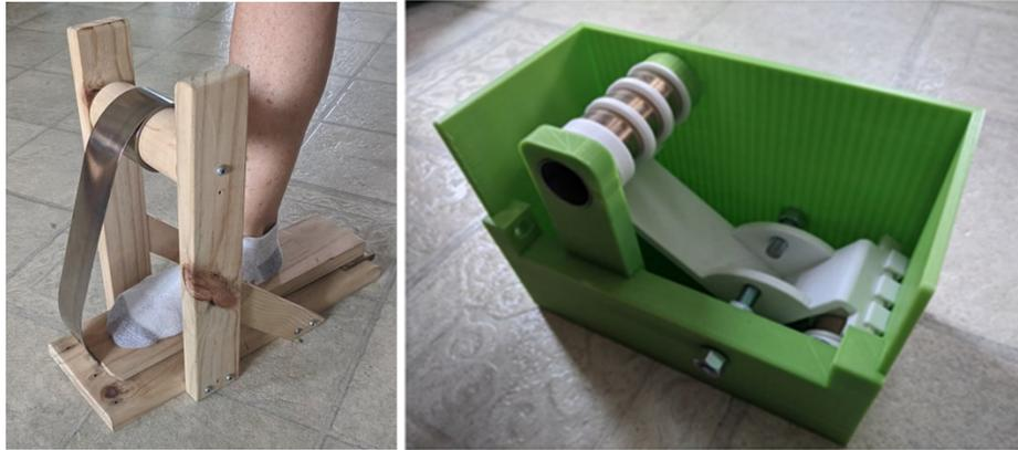
Figure 3.1 : Functional validation prototypes. A) Model for spring validation;
