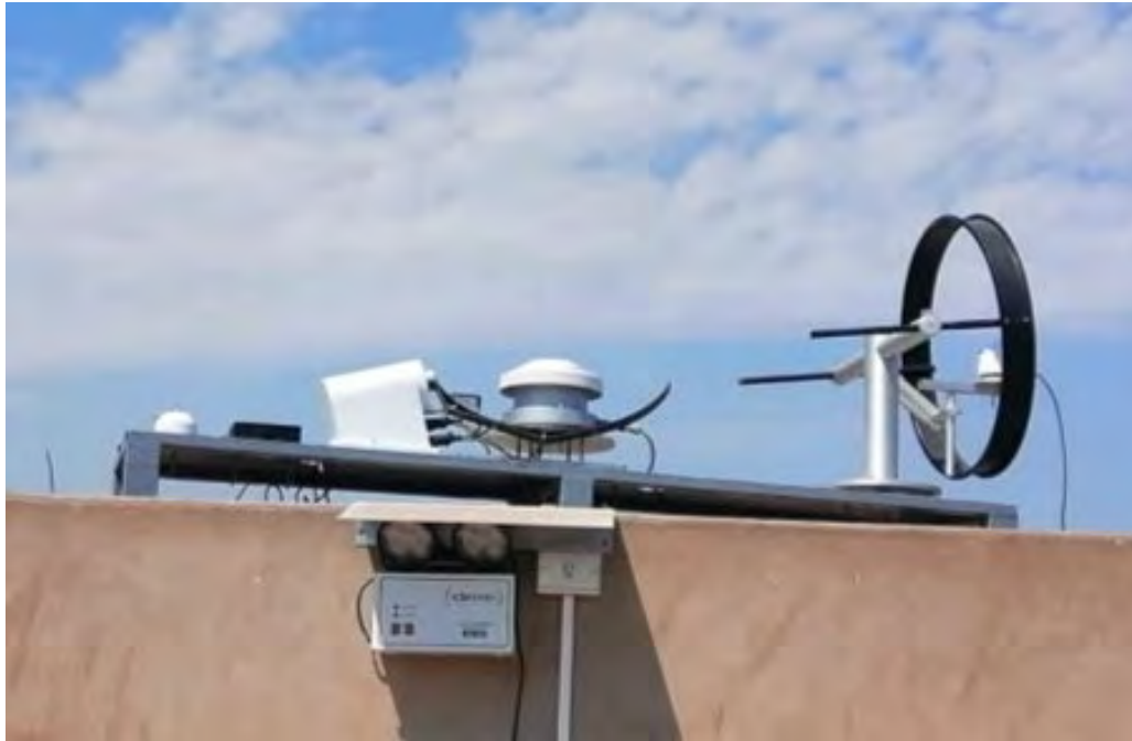
Figure 5.3: Diffuse horizontal measurement systems of the solar spectrum and irradiance.
