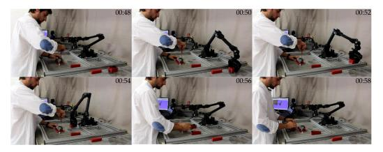
Figure 9. Video frames of the robot being automatically triggered to pick the wheel box and place it on the HWS (task R2) while the screwing task performed by the human is in progress (task H4). The video can be seen in the Supplementary Materials.
