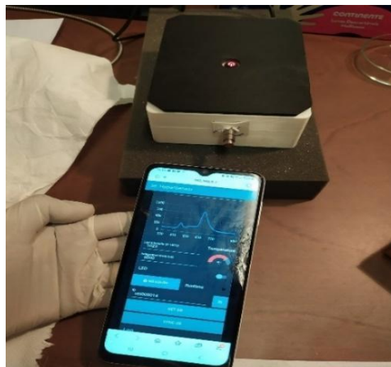
Figure 2. PoC device: Spectrometer system controlled by IoT software in the mobile phone.
