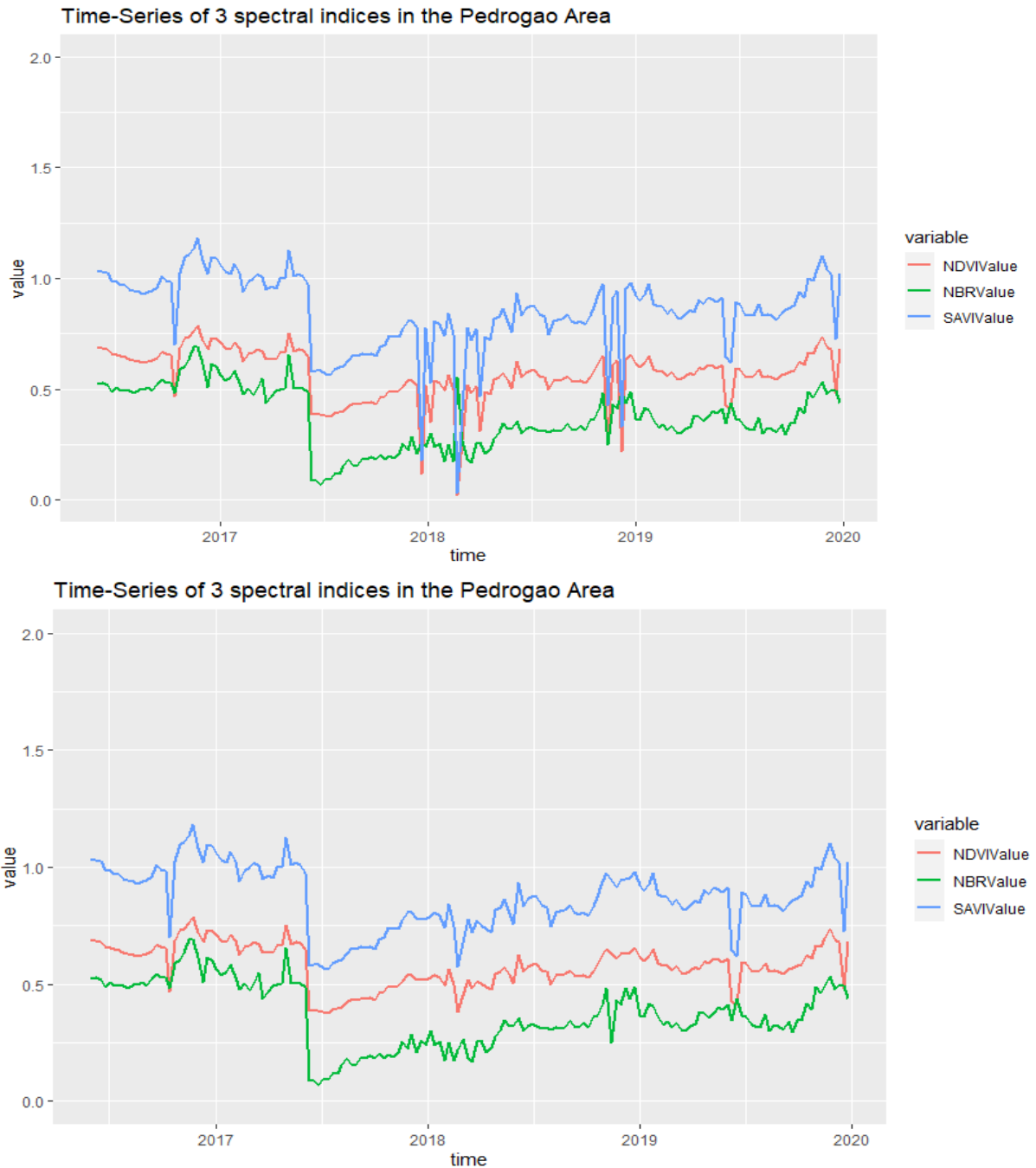
Figure 10 non-Smoothed (top) and Smoothed (bottom) Time-Series of the Pedrogão Área for three spectral indexes
