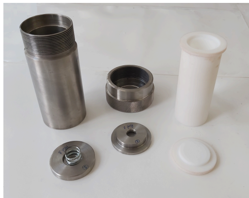
FIGURE 2.1: Teflon recipient and the stainless-steel autoclave used to synthesize the photoanodes through hydrothermal method.
