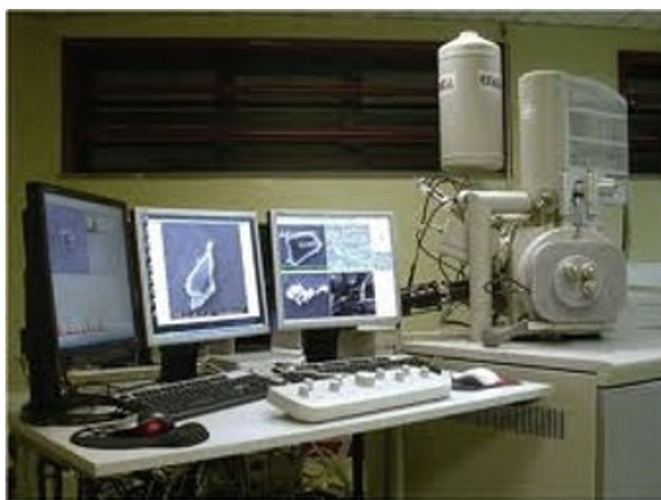
FIGURE 2.7: Scanning Electron Microscope, FEI Quanta 400FEG Field Emission, at CEMUP.
