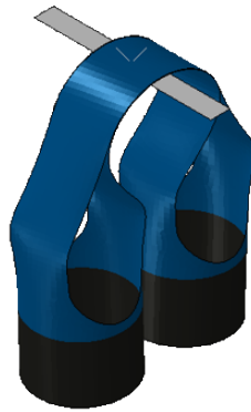
Figure 4.10: Representation of the elastic hinge specimen in a folded configuration.
