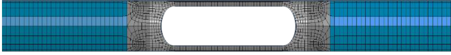
Figure 3.3: Highlight the different regions considered in the structural model. Each region is represented with a different colour (blue, dark grey and light grey) and has a different mesh size.
