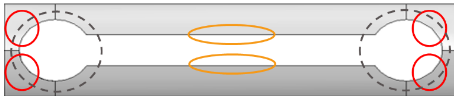
Figure 3.12: Highlight of the stress concentration zones. The regions marked in red have the largest failure indexes, followed by the orange region.
