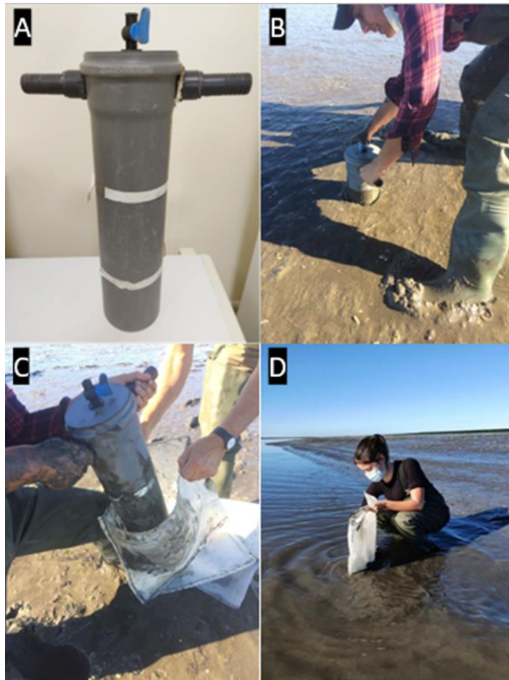
Fig. 4 - (A) The sampling polyethylene core used to survey the benthic communities, (B) sample being removed with core in Bare site, (C) sample being placed in net 0.5mm bag, (D) sample washing in the estuary.
