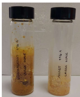
Figure 39 – Resulting extracts from the organic extraction of both supernatant (left) and pellet (right) from the large scale cultures.
