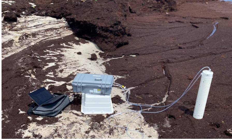
Figure 5. Gas emission data acquisition of shallow Sargassum wrack on beach, using LiCOR trace gas analyzer.
