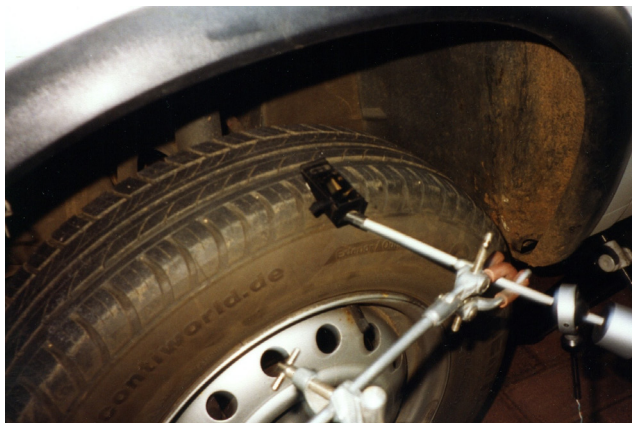
Figure 8.4: Record player stylus fastened to a rigid bracket, touching the tread surface of the tyre
