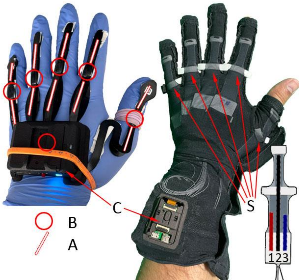
Figure 2. Distribution of the sensors in the Manus Prime II VR gloves (left) and the MoCap Pro Gloves (right). A—IMU; B—Rigid sensors; C—Bluetooth communication controller; S—Stretch sensors that measure the bend and splay of each finger.
