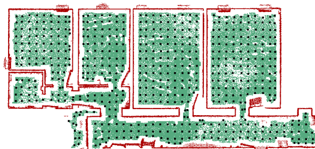
Figure 8. Node distribution in case study 1 for PnRM. Colour code: nodes in black, obstacles in red and navigable floor in green.
