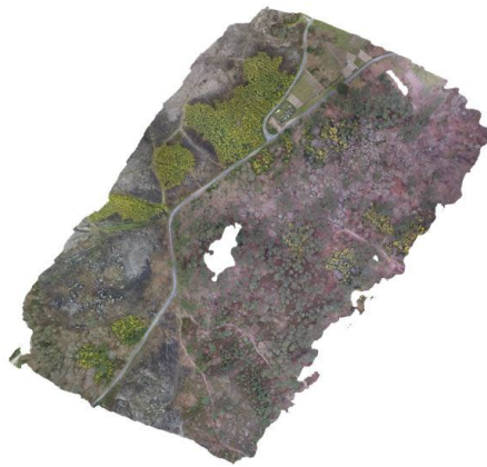
Figure 4 Resulting orthomosaic of the photogrammetric survey based on UAV
