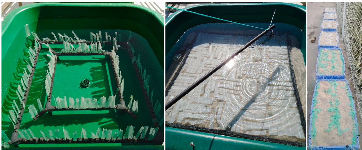
Fig. 1. From left to right: PEL- Samples (beige) are mounted on the PVC test frame, leaving the complete surface area exposed to environmental influences. BEN- Samples (white) are introduced in alternating groups into the system. Three layers of mesh underneath and three layers of mesh on top of the samples secure sample position and contact with the sediment. A frame is used to tighten the mesh. The outflow diameter is extended to 0.196 m 2 surface to prevent clogging. LIT - Four rows of samples are introduced onto the natural beach sand. Samples are mounted to the holding device on one side, allowing movement due to wind.
