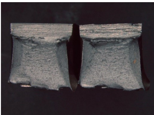
Figure 3.42 Visual inspection of fracture surfaces of the tested Charpy specimens for a) the OM weld, b) the UM weld, c) the OM-UM weld, d) the UM-OM weld and e) the base material.
