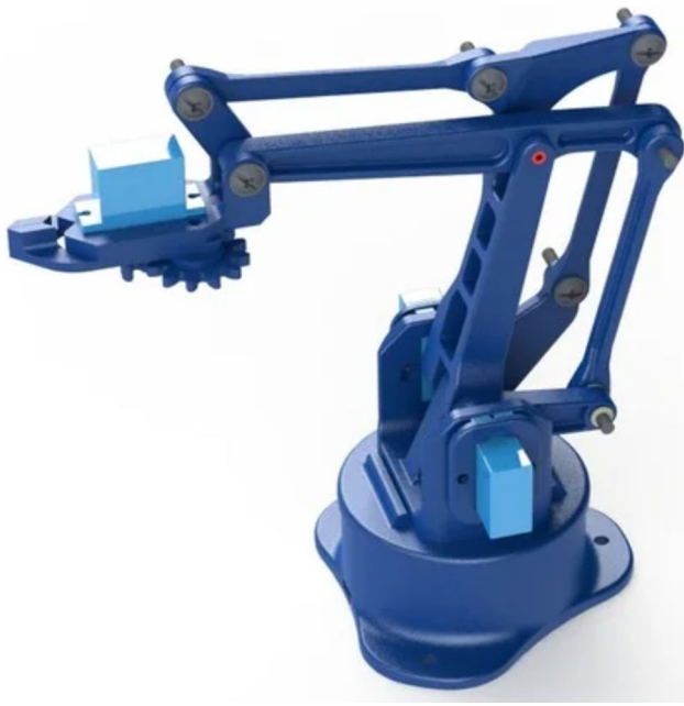
Fig. 2 Representation of the 4-DOF 3D printable robotic arm model
