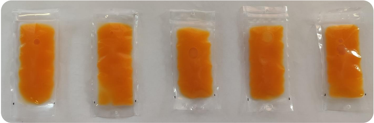
Figure E1. Images of egg yolk samples packaged after each treatment. From left to right: raw egg yolk, egg yolk treated by commercial thermal pasteurization (60 °C/6.2 min), shorter thermal pasteurization (60 °C/3 min), combined treatments at 50 MPa/5 min – 60 °C/3 min and 90 MPa/5 min – 60 °C/3 min.
