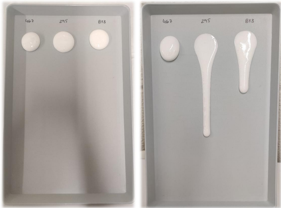
Figure D6. Images of meringue dough prepared with treated and non-treated egg white and its consistency (on an inclined plane, 45 °). From left to right: 467 – meringue batter produced with non-treated EW; 295 – meringue batter produced with EW treated at 55.6 °C/6.2 min; 813 –meringue batter produced with EW treated at 90 MPa/5 min followed by 55 °C/3 min.
