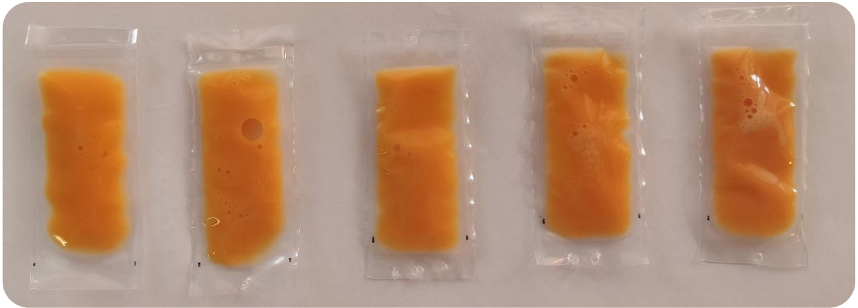
Figure F1. Images of whole egg samples packaged after each treatment. From left to right: raw whole egg, whole egg treated by commercial thermal pasteurization (60 °C/3.5 min), shorter thermal pasteurization (60 °C/1.75 min), combined treatments at 50 MPa/5 min – 60 °C/1.75 min and 200 MPa/5 min – 60 °C/1.75 min.
