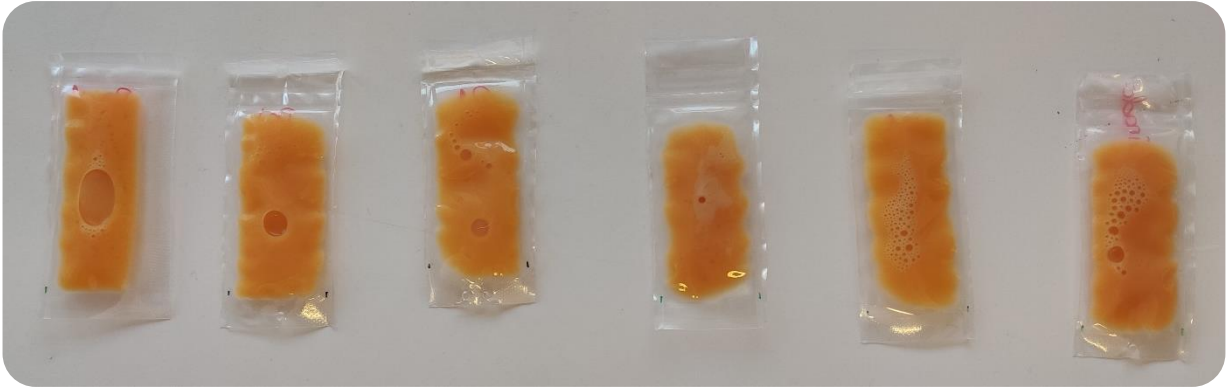
Figure G1. Images of whole egg samples packaged after each treatment. From left to right: raw whole egg, whole egg treated by commercial thermal pasteurization (60 °C/3.5 min), shorter thermal pasteurization (60 °C/1.75 min), moderate pressure (160 MPa/5 min), ultrasound (50 % amplitude/1 min), and combined treatment (160 MPa/5 min – 50 % amplitude/1 min – 60 °C/1.75 min).
