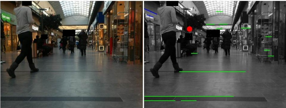
Fig. 6.6. An image captured by the smartphone on the left and after processing using the visual gyroscope algorithm on the right. The lines found from the image are classified and colored, the ones in the direction of propagation and used for the vanishing point calculation being in blue. The central vanishing point is shown as a red dot.
