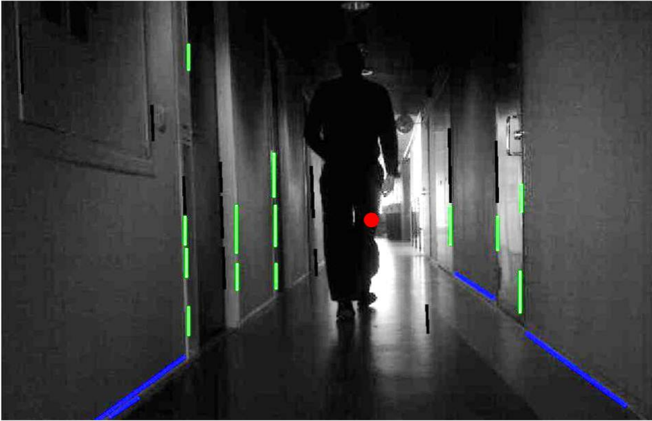
Fig. 4.5. Calculation of the central vanishing point is largely tolerant to dynamic objects in the scene.
