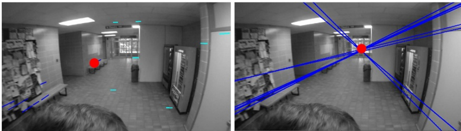
Fig. 6.18. Vanishing point detection in an environment suffering from low lighting and non-orthogonal lines, on the left using the visual gyroscope presented in Chapter 4, and on the right using the visual gyroscope based on Probabilistic Hough Transform.
