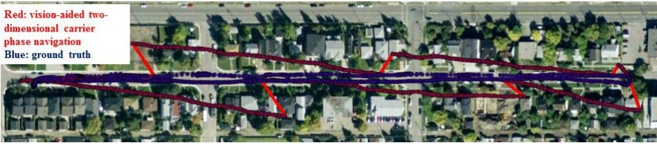
Fig. 7.2. Position solution verification using vision-aided carrier phase navigation (position red dot, path red line) and compared to ground truth (blue) in a sub-urban environment in Calgary, shown in Google Earth.
