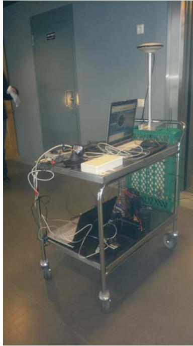
Fig. 6.1. Equipment setup for experimenting the vision-aided multi-sensor positioning. The Nokia N8 phone acquiring the images was attached to a holder in the front of the cart. The GNSS antenna is that of the NovAtel SPAN reference system.
