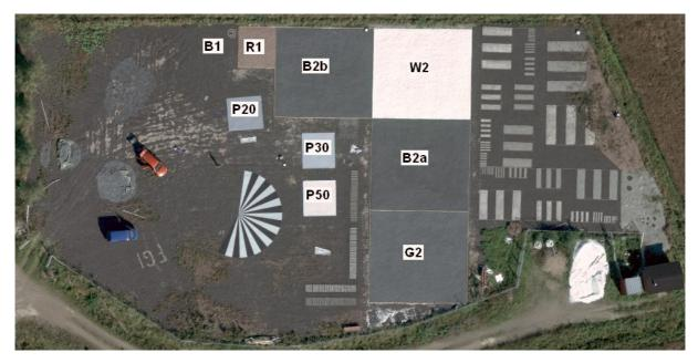
Figure 7. The modernized Metsähovi image quality test field in 2008 during the 1.9.2008 DMC campaign. For abbreviations, see Table 3 (from II).
