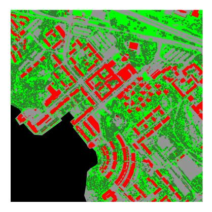
Figure 13. The land cover classification results obtained using laser scanner and aerial image data. The figure shows a 900 m  $\times$  900 m part of the study area used in VI.
