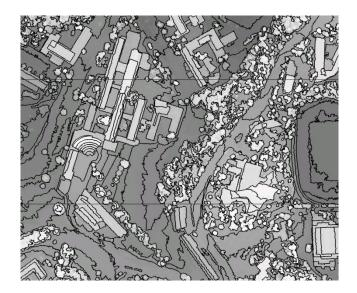
Figure 1. Segmentation of a DSM derived from laser scanner data (from II).
