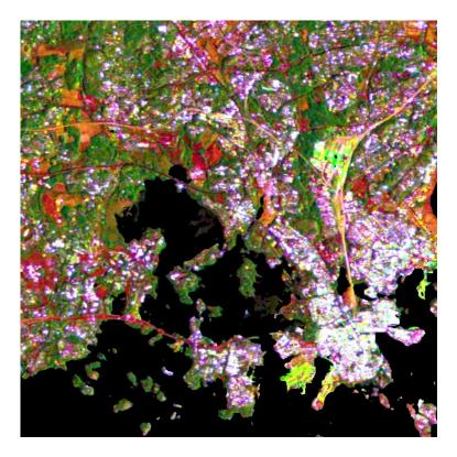
**Figure 3.** An example of a multitemporal interferometric SAR dataset (from I; SAR data  $\bigcirc$  M. Engdahl and ESA AO3-277). The channels of the colour image: temporal average of Tandem coherence images in red, temporal average of backscatter intensity images in green, and average of two long-time coherence images in blue. The figure shows a 12 km × 12 km subarea of the dataset.
