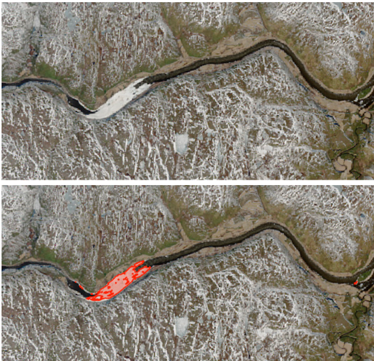
Figure 13. Identification of a possible site for ice dam formation (Landsat-8 2018-05-13).
