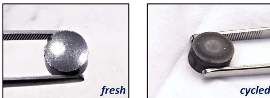
Fig. 4 – Images of a pellet before the first desorption (left) and after spectral signal loss due to cycling (right), as shown in Fig. 3.
