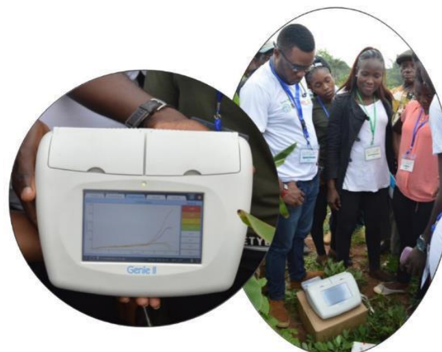
Step - 3. Reaction incubation and real time detection (10 – 15 min)
