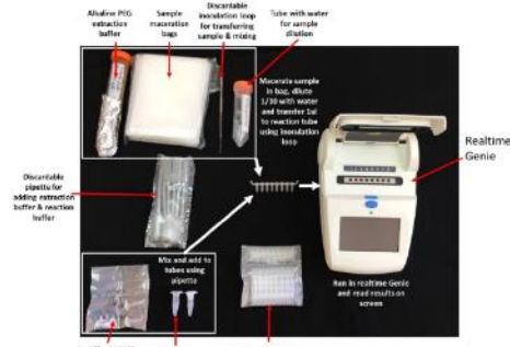
Figure 2 Components of prototype field LAMP kit for detection of sweetpotato viruses.
