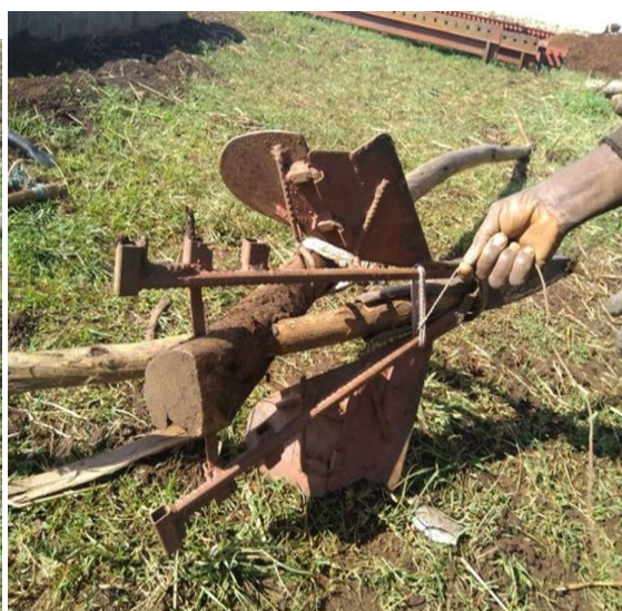
Winged Berken plow for deep tillage in Kulumsa (Oromia region), photo credit by Abera Assefa
