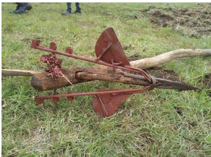
Berken plow for deep tillage in Kulumsa (Oromia region), photo credit by Abera Assefa
