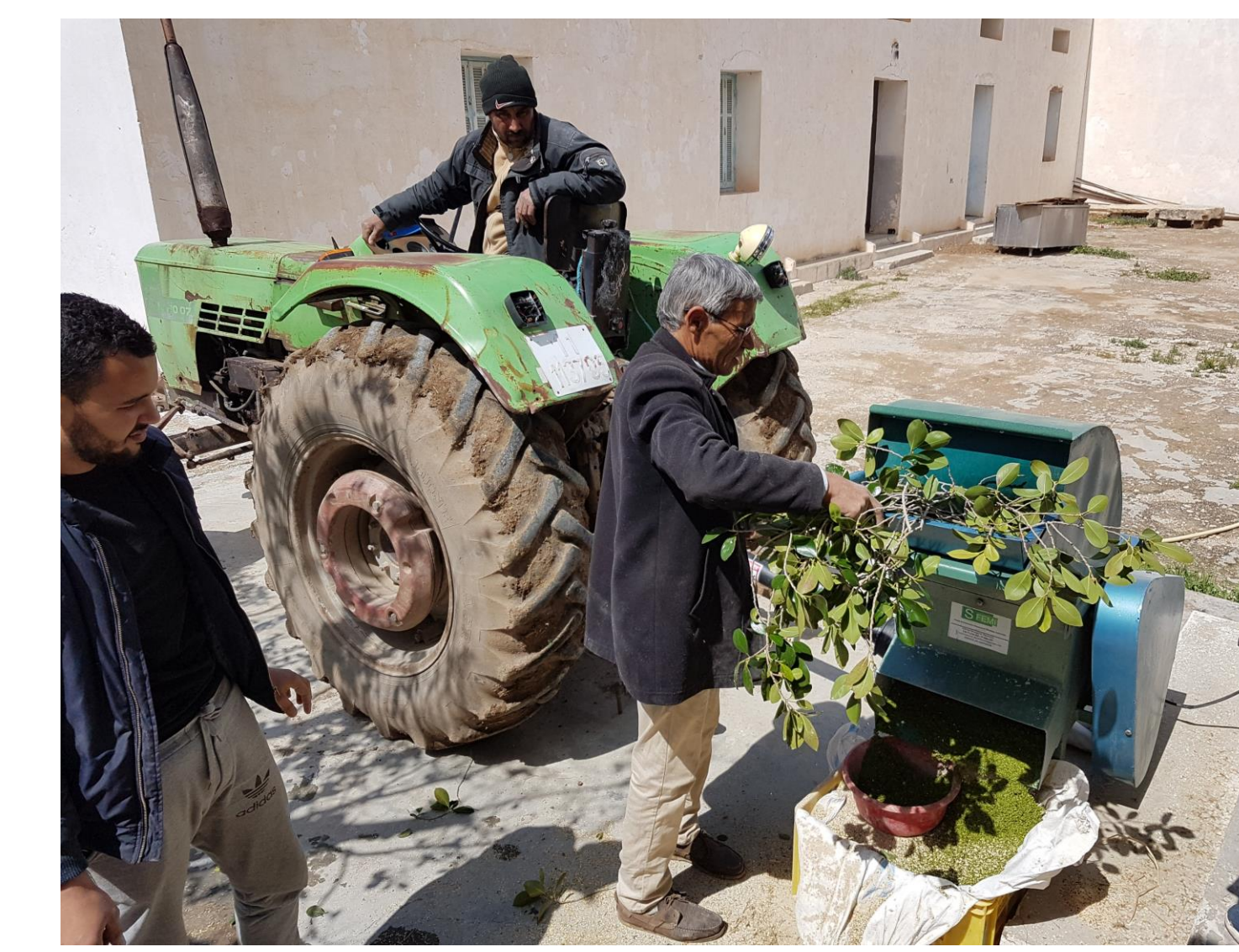
Mobile grinder chopping organic material for compost and improved feed digestion
