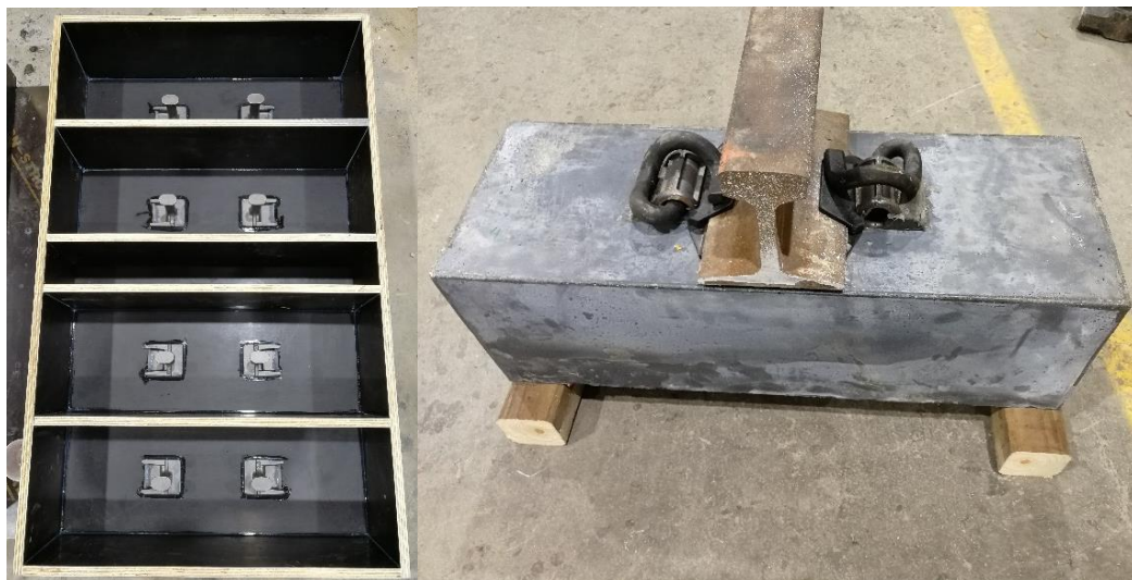
(a) moulds with shoulders
