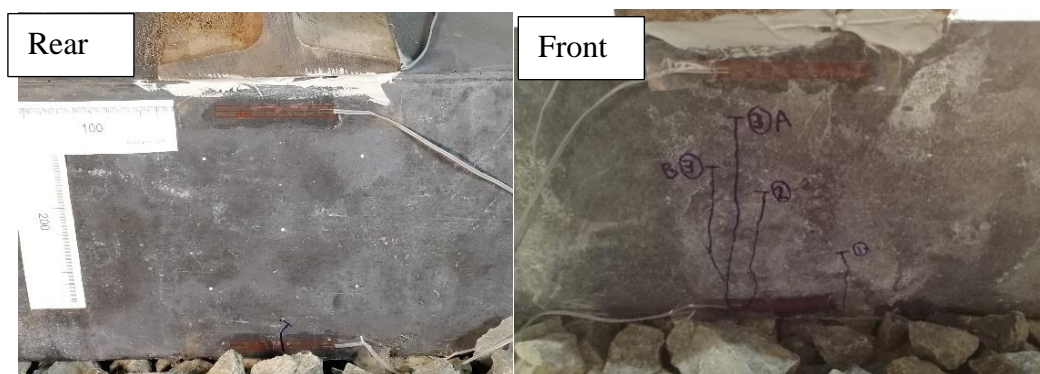
(a) after Drop 5 (the first cracks)
