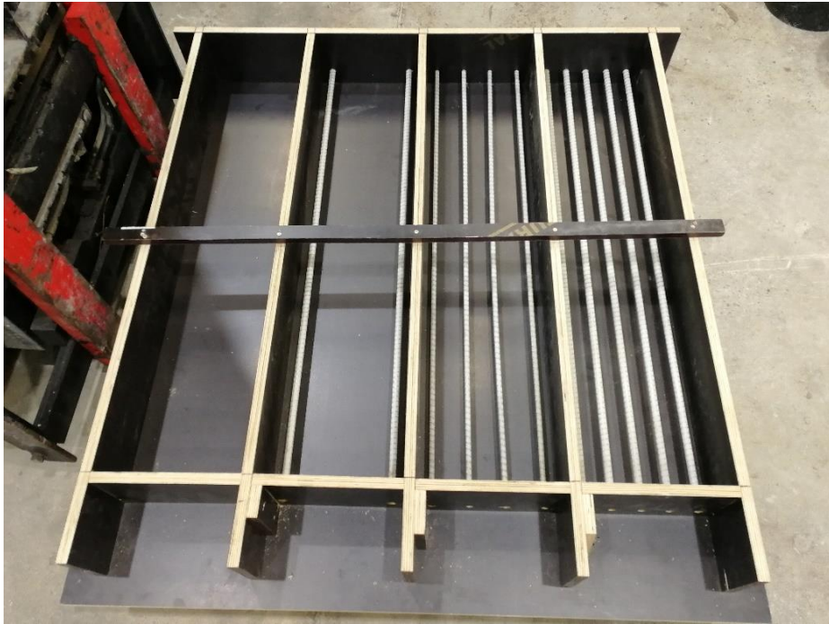
Figure 6.2 A view of the moulds and the GFRP bars for making the low-height UHP-FRC sleepers
