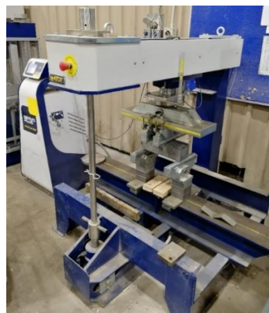
(b) 100 kN MATEST test rig for flexural testing of UHP-FRC samples
