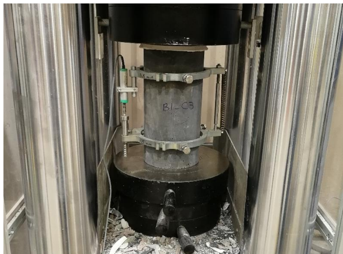
Figure 3.13 Determination of the modulus of elasticity of the optimal UHP-FRC mix in congruence with 1012.17 (AS-1012.17, 1997)
