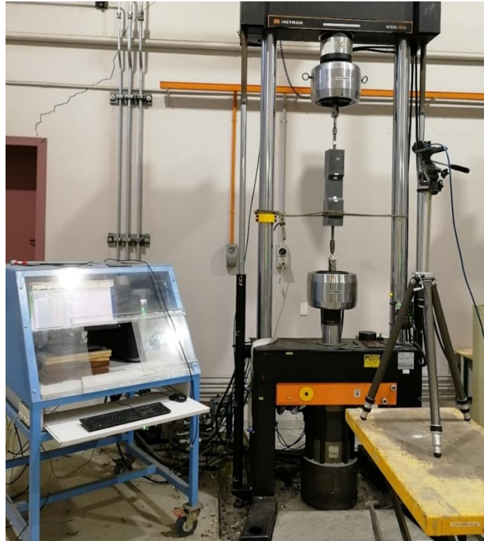
Figure 7.15 Direct tensile test (DTT) set-up
