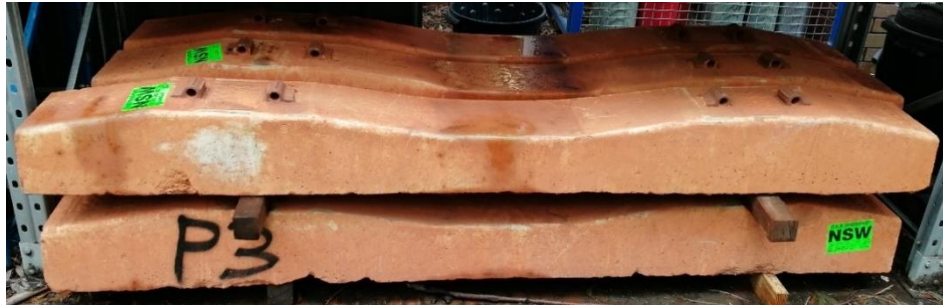
Figure A.1 A view of the heavy-haul PSC sleepers
