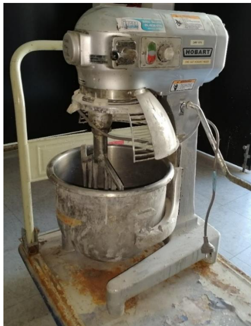
Figure 3.3 The Hobart mixer used for mixing the trial UHP-FRC mixes
