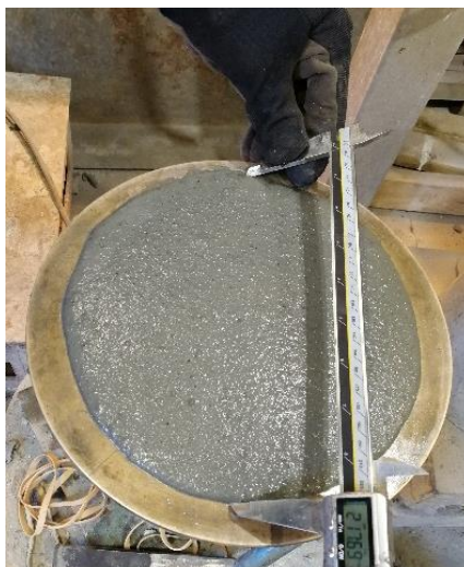
Figure 3.4 Flow table testing of the UHP-FRC mixes in congruence with ASTM C230/C230M (C230/C230M, 1998)
