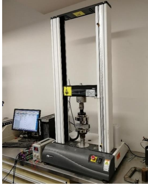
(b) the 30 kN Instron test rig for flexural testing of the UHP-FRC samples
