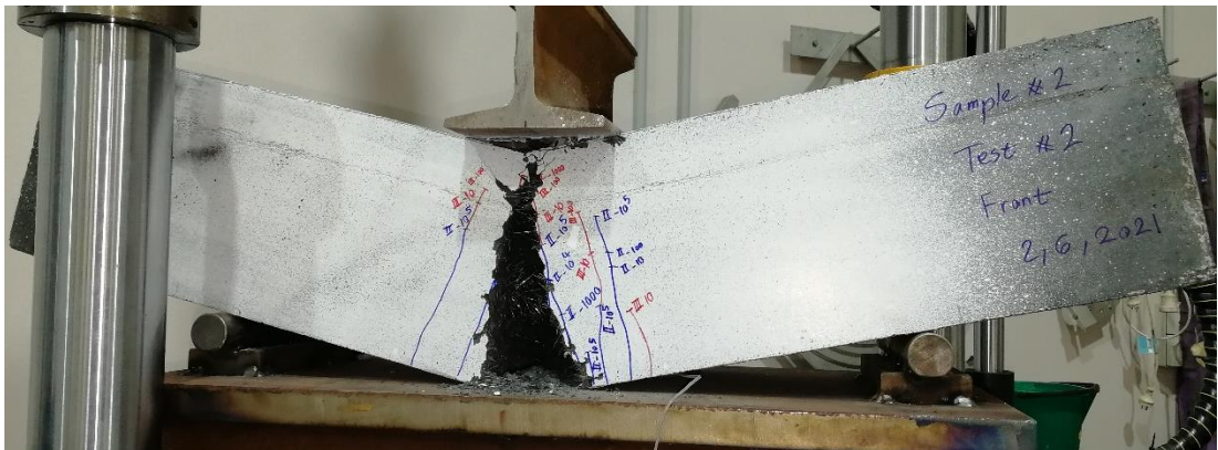
Figure 4.28 Ultimate failure of sample S2-F2
