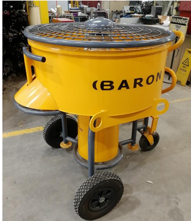
Figure 4.2 The 300-litre pan mixer for producing the UHP-FRC mixes
