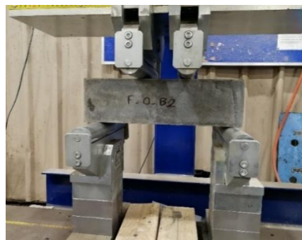
(a) prismatic samples of 100x100x350 (mm) for flexural testing
