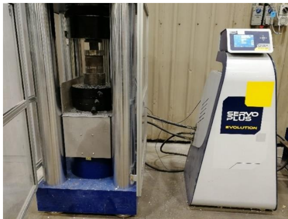
(b) 3000 kN MATEST test rig for compression testing of the UHP-FRC samples
