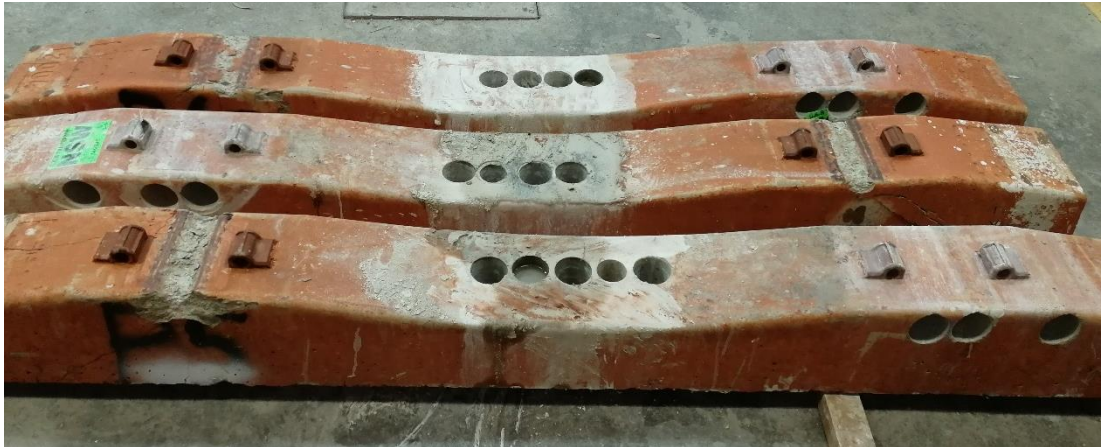
Figure A.7 A view of the horizontal and vertical core holes
