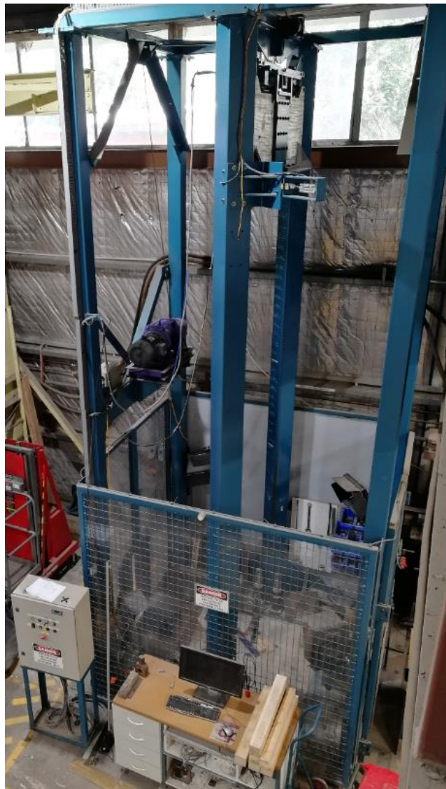
Figure 5.1 The drop-hammer impact testing machine at the University of Wollongong
