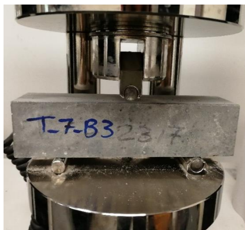
(a) prismatic UHP-FRC sample of 40x40x160 (mm) for flexural testing
