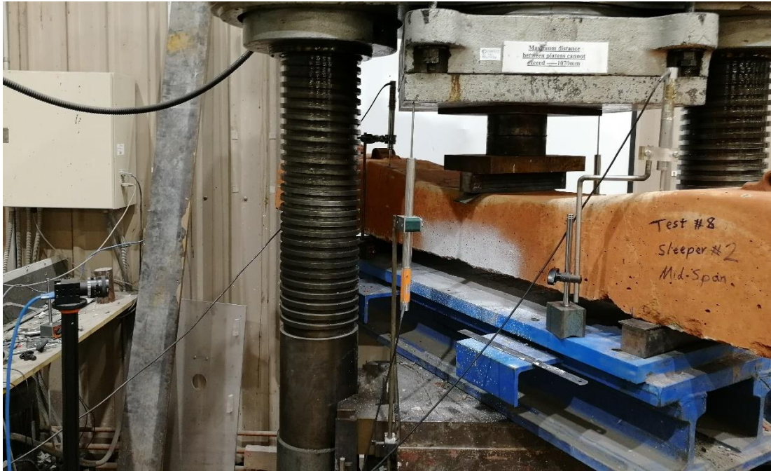
Figure A.5 The 3-point bending test set-up for determining the prestressing force
