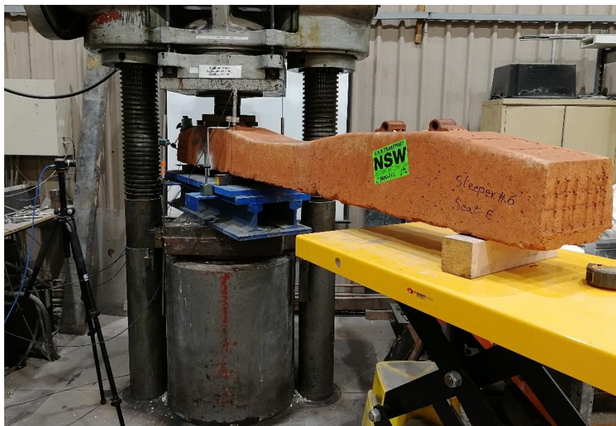
Figure A.2 The positive moment rail-seat test set-up of the heavy-haul PSC sleepers
