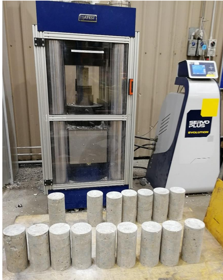
Figure A.8 The universal compression testing of the core samples
