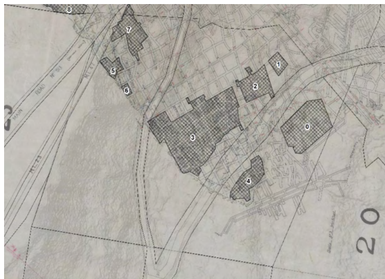
Figure 10: Excelsior I, II and B Collieries board and pillar operations in the vicinity of Bulli Pass
