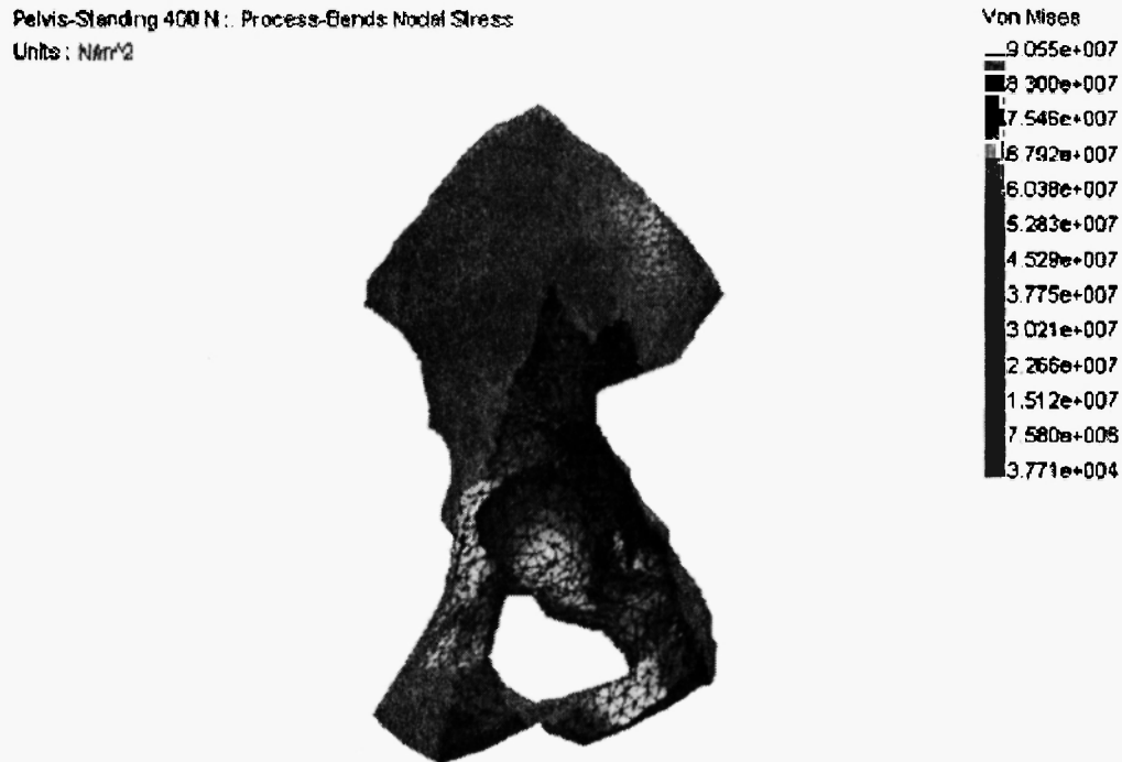
Fig. 8: Sample finite element analysis of a hip bone with 400N force applied /29/.
