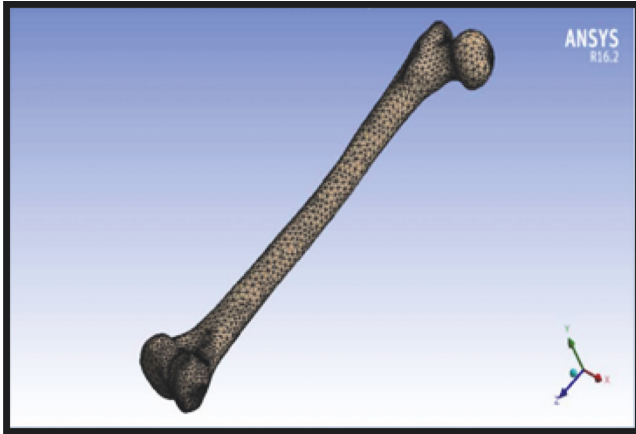
FIGURE 10: Meshing with tetrahedral elements.
