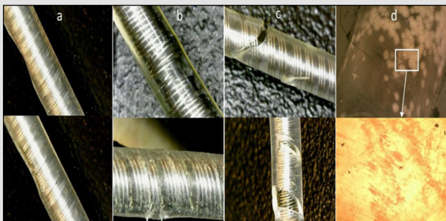
Figure 6: Samples of Lead Damage Modes, (a) Abrasion, (b) Coil Damage, (c) Insulation Defect, (d) Discoloration.
