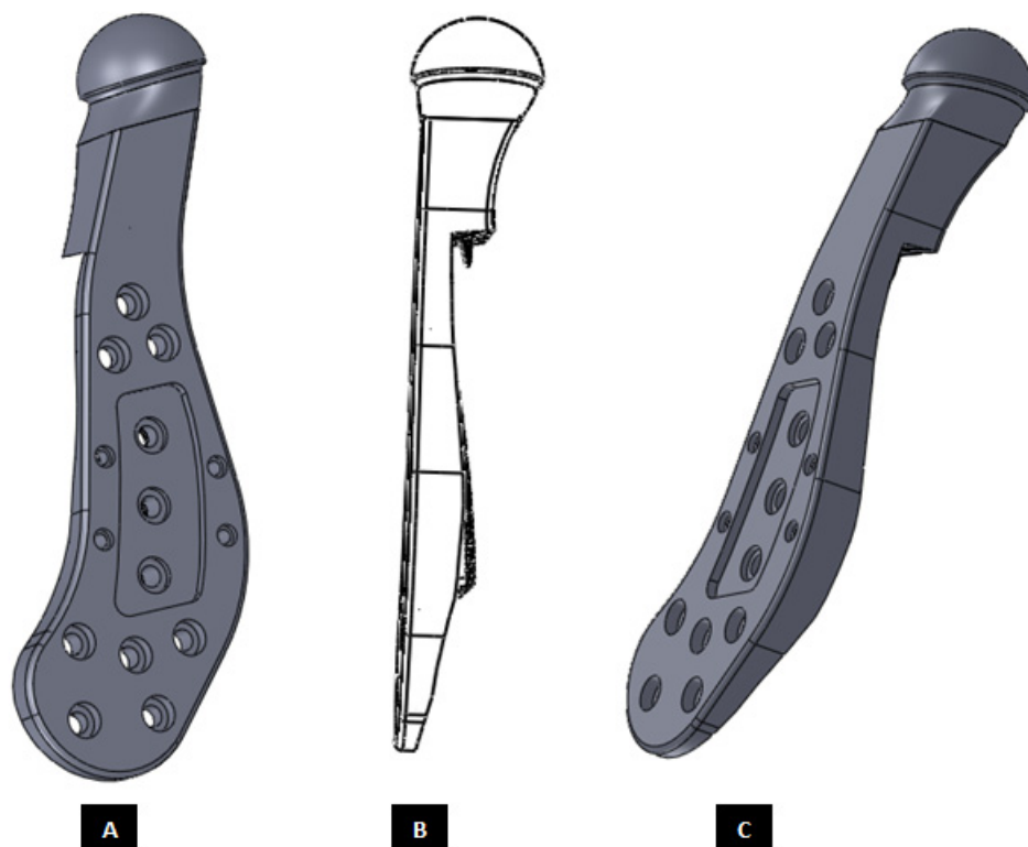
Figure 12. Modification and refinement of custom-designed condylar/ramus component shown in Figures 9 and 11. (A,C) Show pre-drilled screw holes and a groove in the lateral surface of implant. As shown in (C), lateral surface of the device is flat and medial surface is shaped to match the host bone geometry. (B) Shows a perforated notch each protruding from the medial surface of the ramus and inferior surface of the implant collar/neck.
