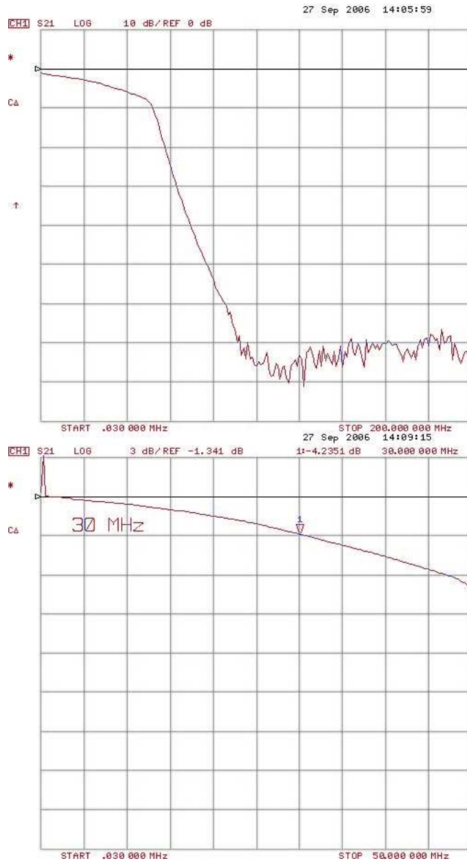
Figure 4.10: MON1 Output to ADC1 Input up to 200MHz, 10dB/Div. (Top) and up to 50 MHz, 3dB/Div. (Bottom) of the DC-Coupled Board.
