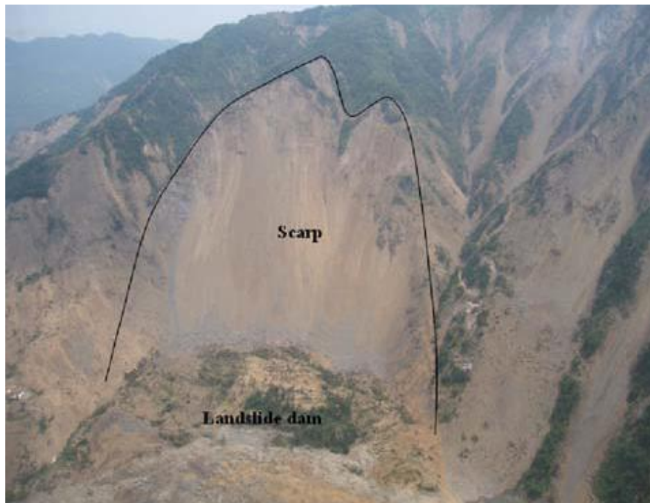
Figure 12: Helicopter view of the Tangjiashan landslide dam and scarp (Xu et al., 2009).
