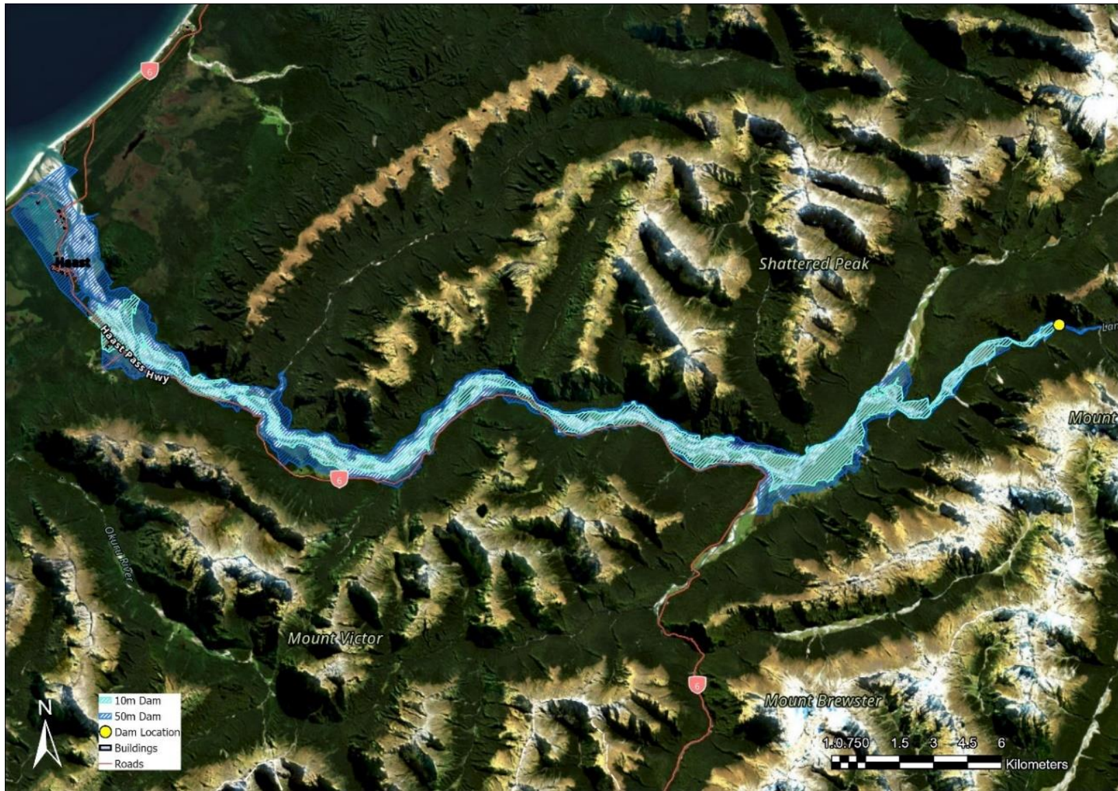
Figure 47- Outburst flood inundation map for the Haast Landsborough catchment at 10 m and 50 m landslide dam heights showing downstream exposure.
