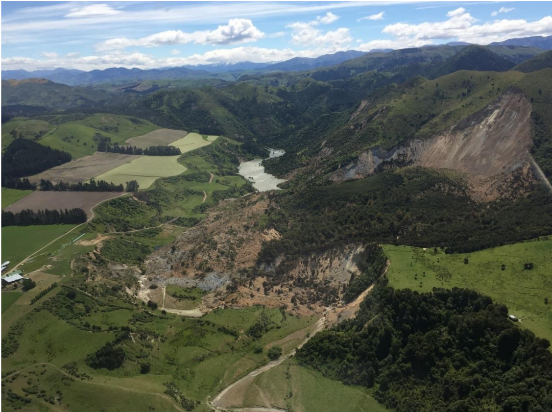
Figure 15 - Landslide dam on the Leader River. The landslide is a slump/block slide in a siltstone unit. The landslide dam overtopped and partially breached on the 15 th of November 2016 within 24 hours after the earthquake, with the full breach occurring on the 13 th – 14 th of February 2017 (Dellow et al., 2017a).
