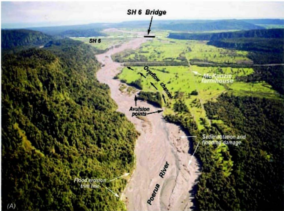
Figure 19- Oblique aerial photos of the Poerua River fan showing the effects of the dam break flood. October 1999, 2 days after the dam breach (Hancox et al., 2005).
