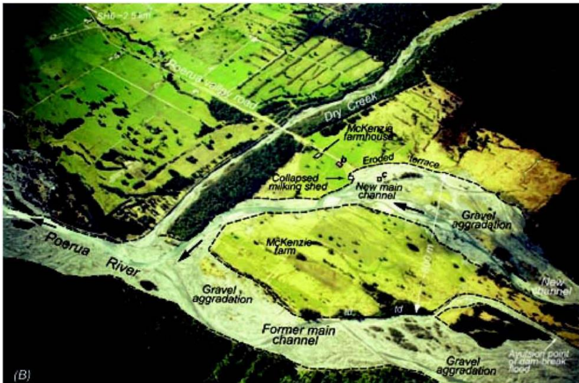
Figure 20- Oblique aerial photos of the Poerua River fan showing the effects of the dam break flood. August 2001, after 22 months of sediment aggradation and erosion (Hancox et al., 2005).
