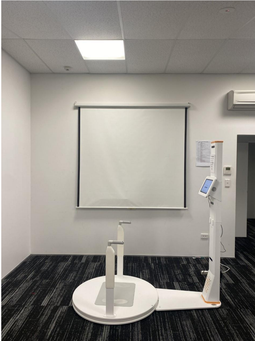
Figure 20. FIT3D® optical scanning device set-up
