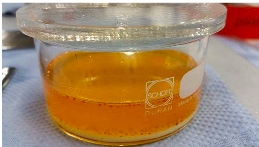
Fig. 3. The fuel after 160 h at 30 V, 80 °C.
