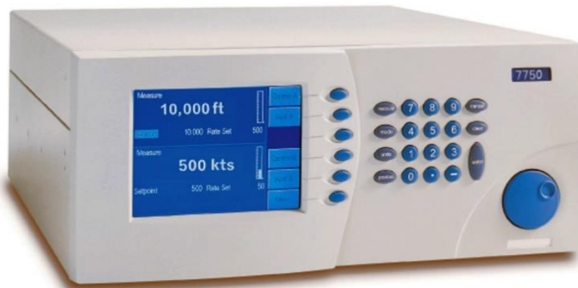
Figure 29: The pressure transfer standard Ruska 7750i which is used for all pressure calibrations of the HALO nose boom sensors.
