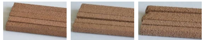
Fig. 2. Conductors of 100% (sample 2.5), 80% (sample 2.3) and 60% (sample 2.1) printing density.
