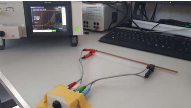
Fig. 4. Hioki IM3570 Impedance Analyzer with probe and Kelvin terminals
