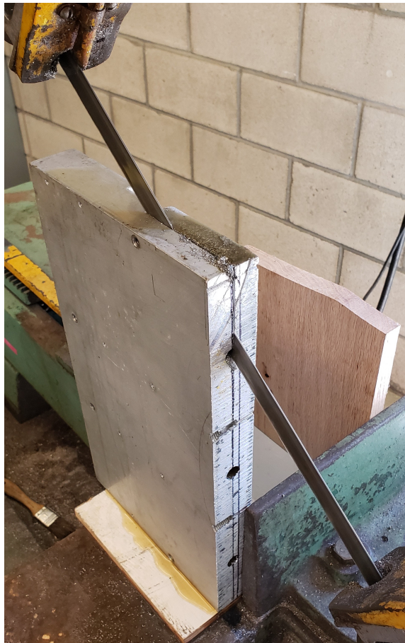
Figure 3.16: Heater plate in the horizontal bandsaw to cut along the thickness
