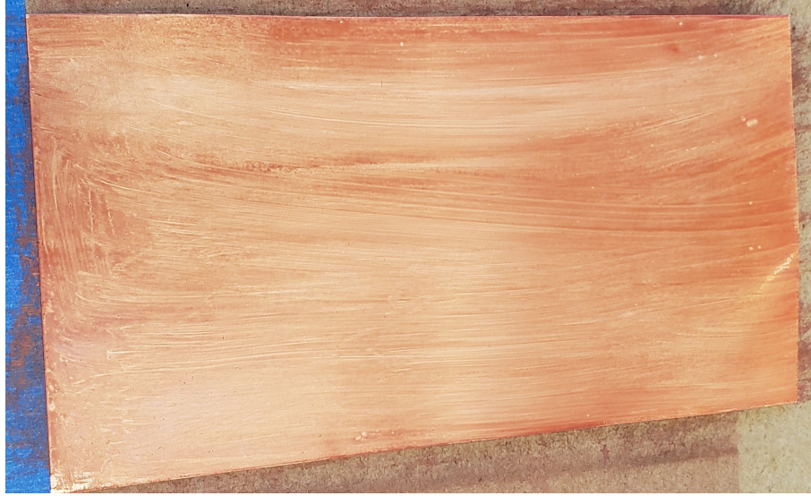
Figure 3.12: Second primer coupon with minimal fisheyes and even, thinner application
