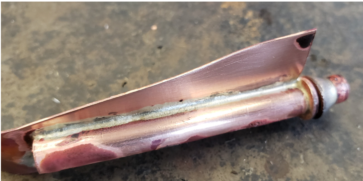
Figure 3.2: 1st brazing coupon with round tubing and thicker copper sheet
