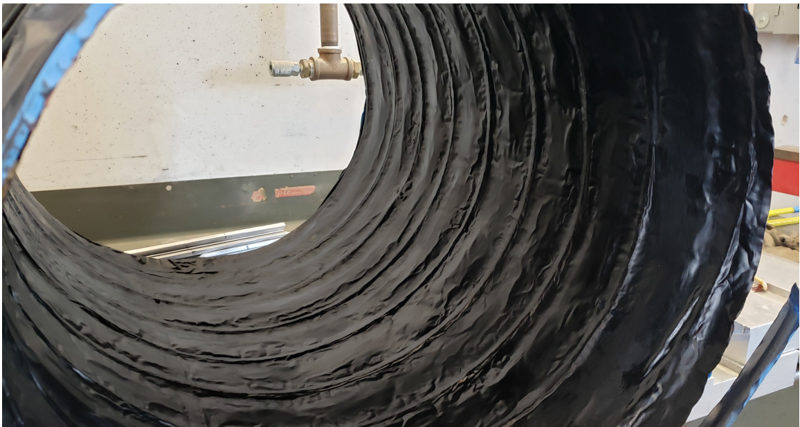
Figure 3.15: Shroud interior after Aeroglaze Z306 application
