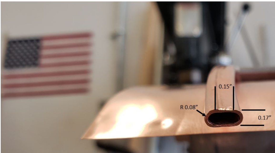
Figure 3.1: Tubing cross section after rolling process
