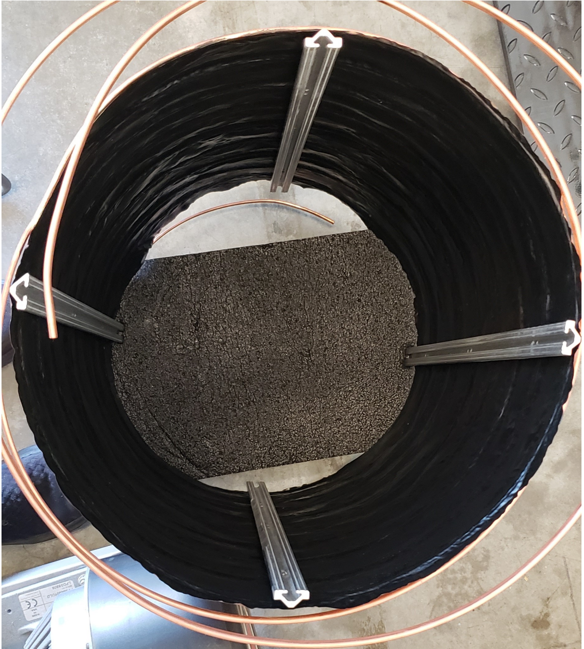
Figure 3.23: Shroud after mounting rails were installed
