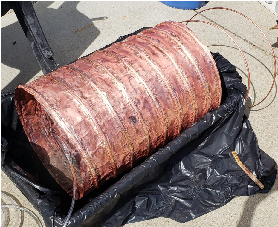
Figure 3.7: Shroud in plastic tub during cleaning with dilute hot citric acid
