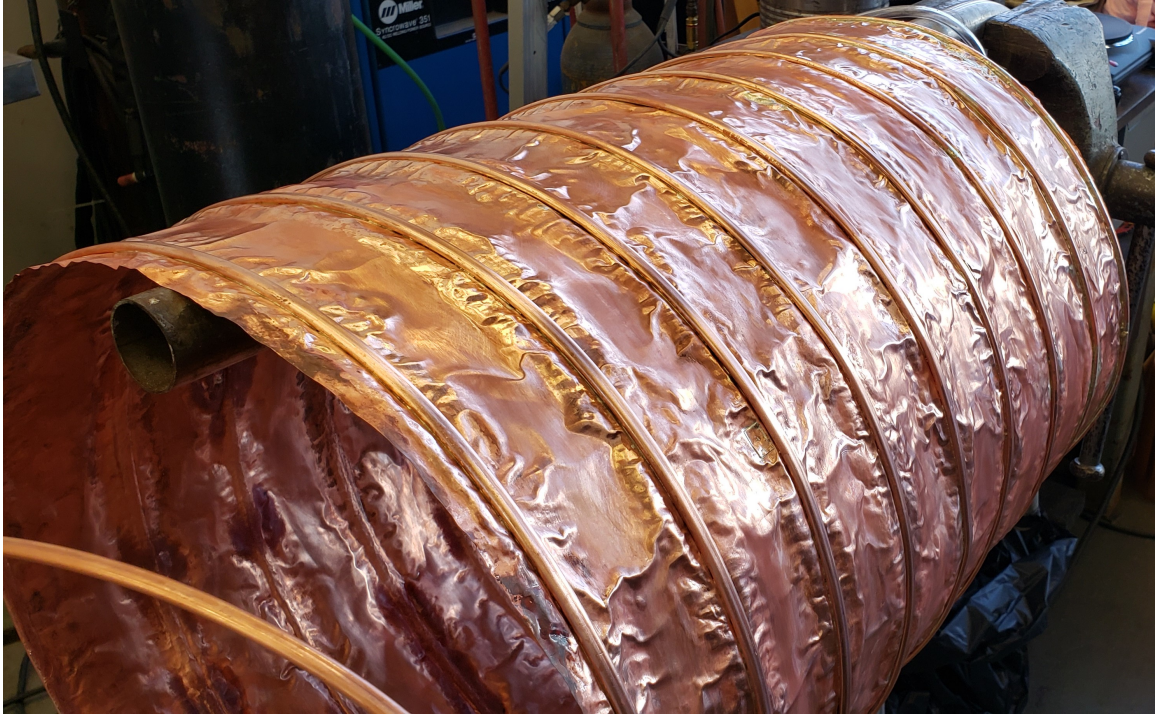
Figure 3.8: Shroud after cleaning process with dilute hot citric acid
