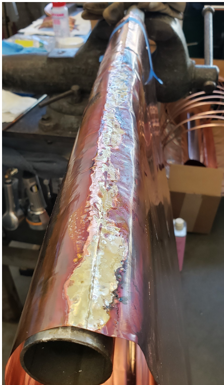
Figure 3.4: Copper sheet during brazing process for cylinder forming
