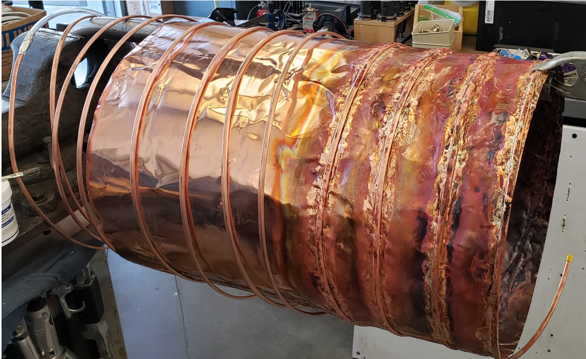
Figure 3.6: Shroud during brazing process
