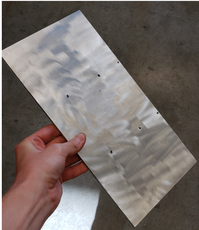
Figure 3.19: Heater plate front face after final machining
