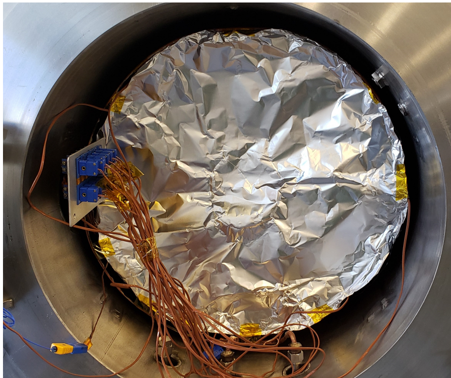
Figure 4.6: Empty test 1 & 2 configuration experimental setup with front foil reflector
