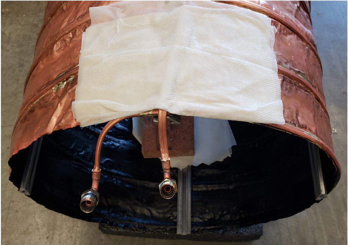
Figure 3.25: Shroud connector brazing setup with wet cooling towels
