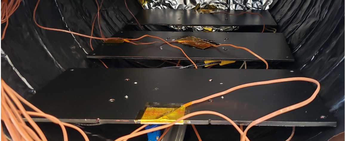
Figure 3.21: Heater plates integrated into the shroud after painting
