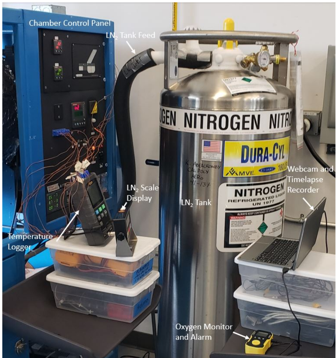
Figure 4.3: Labeled data collection experimental setup
