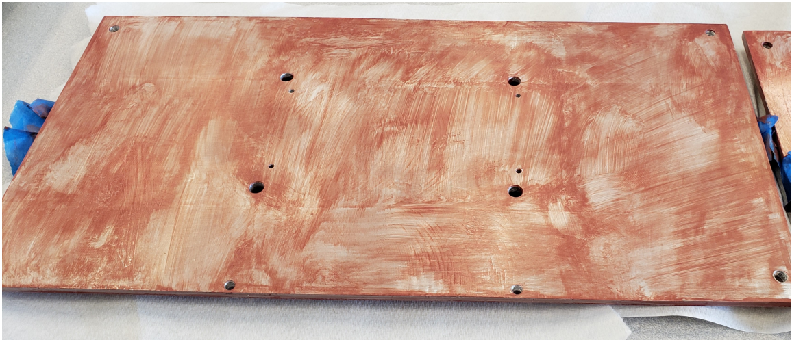
Figure 3.20: Heater plates after primer application with additional mounting holes visible
