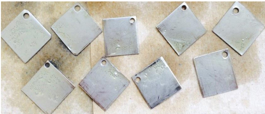
Figure16. Stainless steel coupon pretreated with canola oil.
