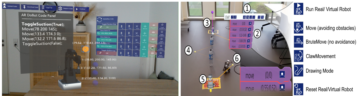
Figure 2. AR programming interface: programming the dobot arm (left) and the Lego NXT robot (right)
