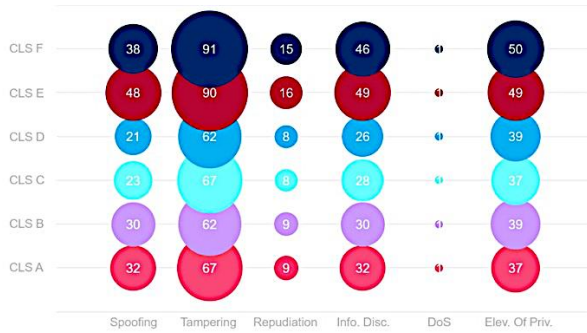
Figure 1: The cumulative attack surface for all six modeled streetlighting systems, mapped to the STRIDE framework.
