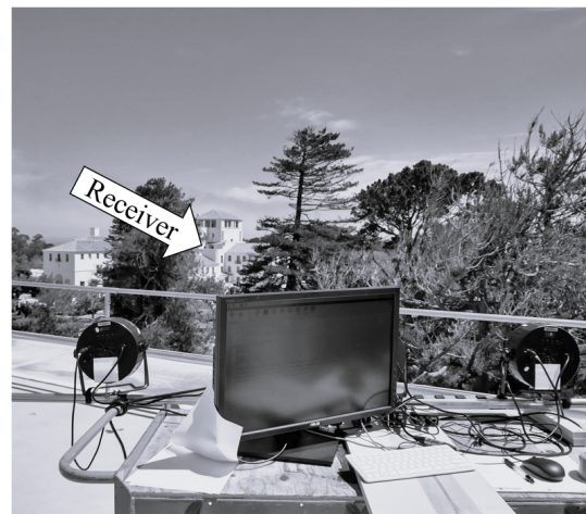
Figure 5. View from transmitter to collector on tower (192 m).
