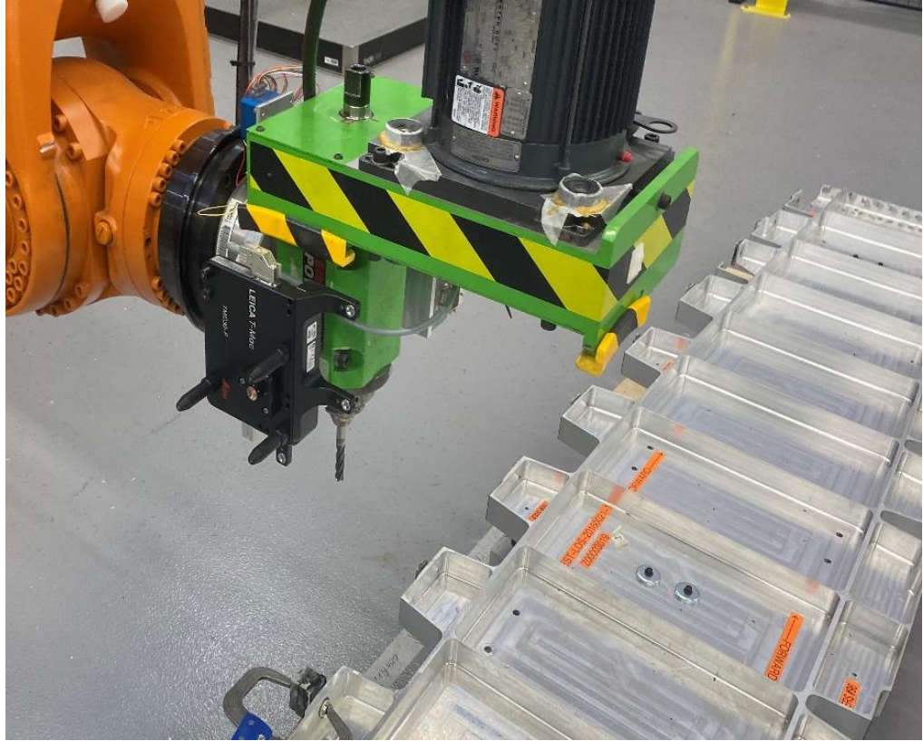
Figure 1.1: Aerospace wing rib with CNC machined thin-walled regions
