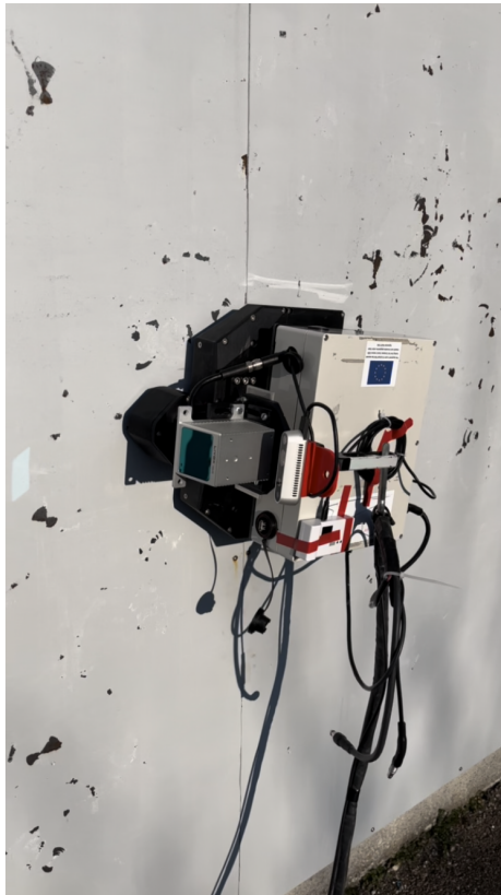
Figure 1.2: An image of the ROBOPLANET Altiscan in action on a vertical surface. The cord attached to the chassis of the crawler is the tether that contains a bundle of transfer cables for data, power, and water supplies.
