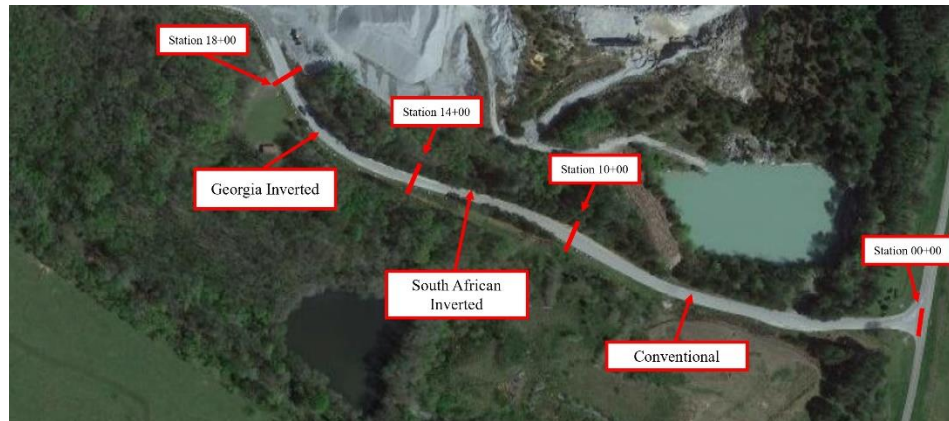
Figure 2.3 Morgan County, GA test sections. Image from Google (n.d. a)
