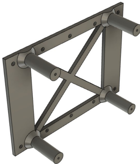
Figure E.3: Robotic Arm Mount. This allows the robotic arm to be mounted to the 2020 Aluminum frame. Rows of holes are for screws which attach the mount to the inside slots of a framing rod. Large standoffs are used to get the arm closer to the turntable. The part is mostly hollow to speed up printing time.
