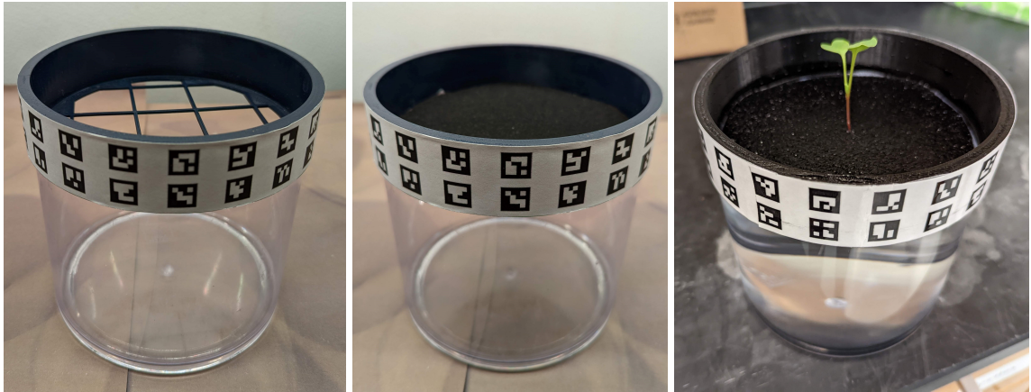
Figure 3.1: Growing Canisters. Left: Canister with net pot. Center: Canister and net pot with felt. Right: Canister with net pot, felt, and growing radish plant.
