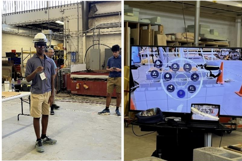
Figure 3 – Student using OHMD to compare as-built wall to REVIT model on the left and view from the OHMD on the right
